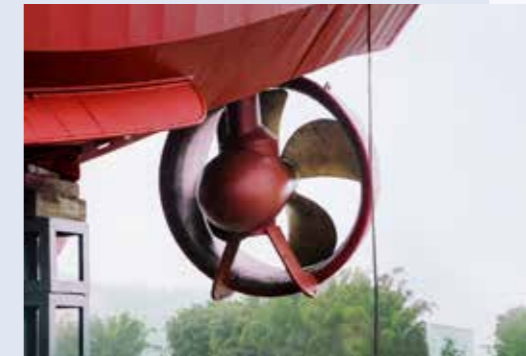
MAINTENANCE can be carried out based on the condition of the propulsion system.
