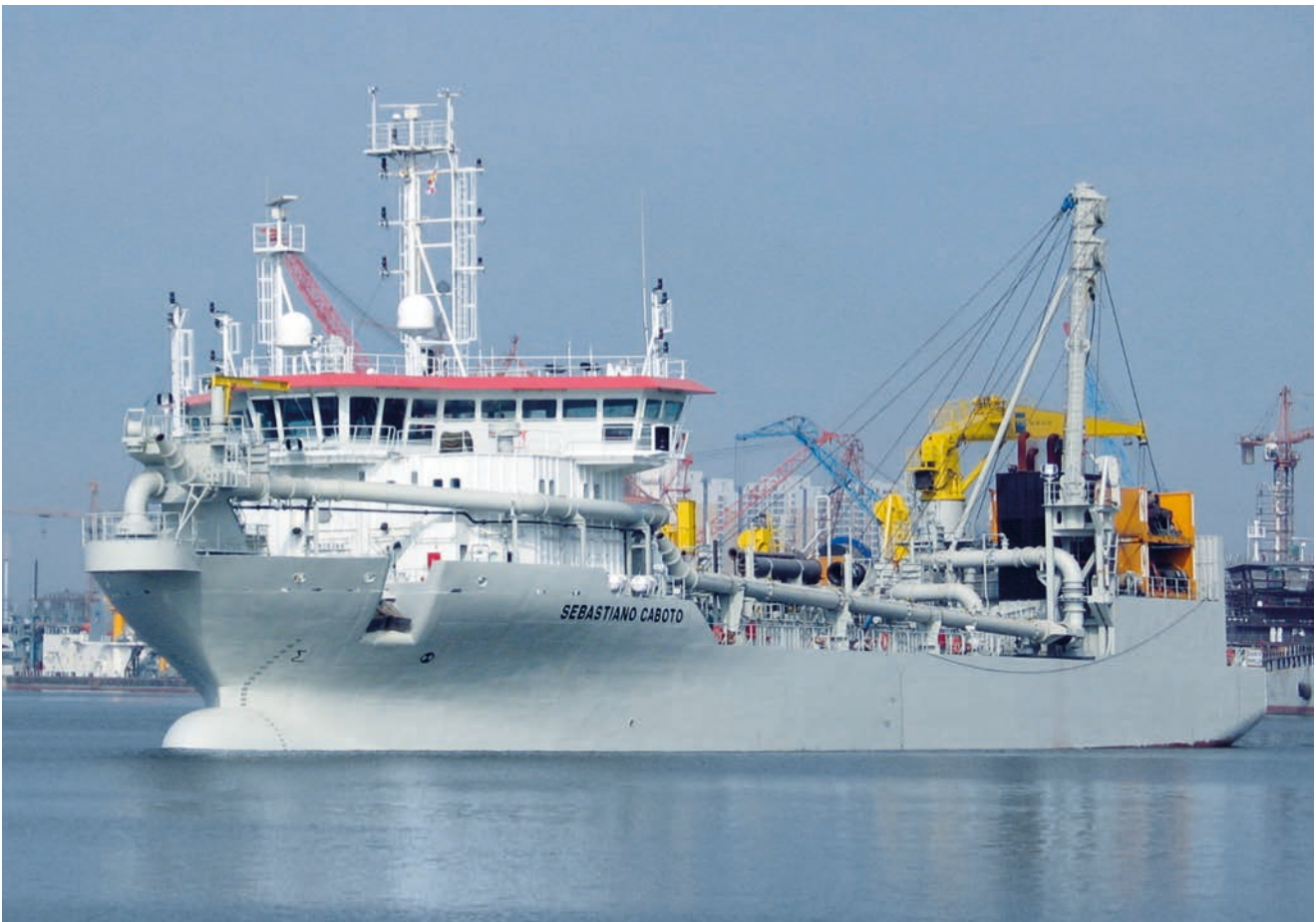
Trailing Suction Hopper Dredger Sebastiano Caboto 2 x SRP 1010 (1000 kW each)
