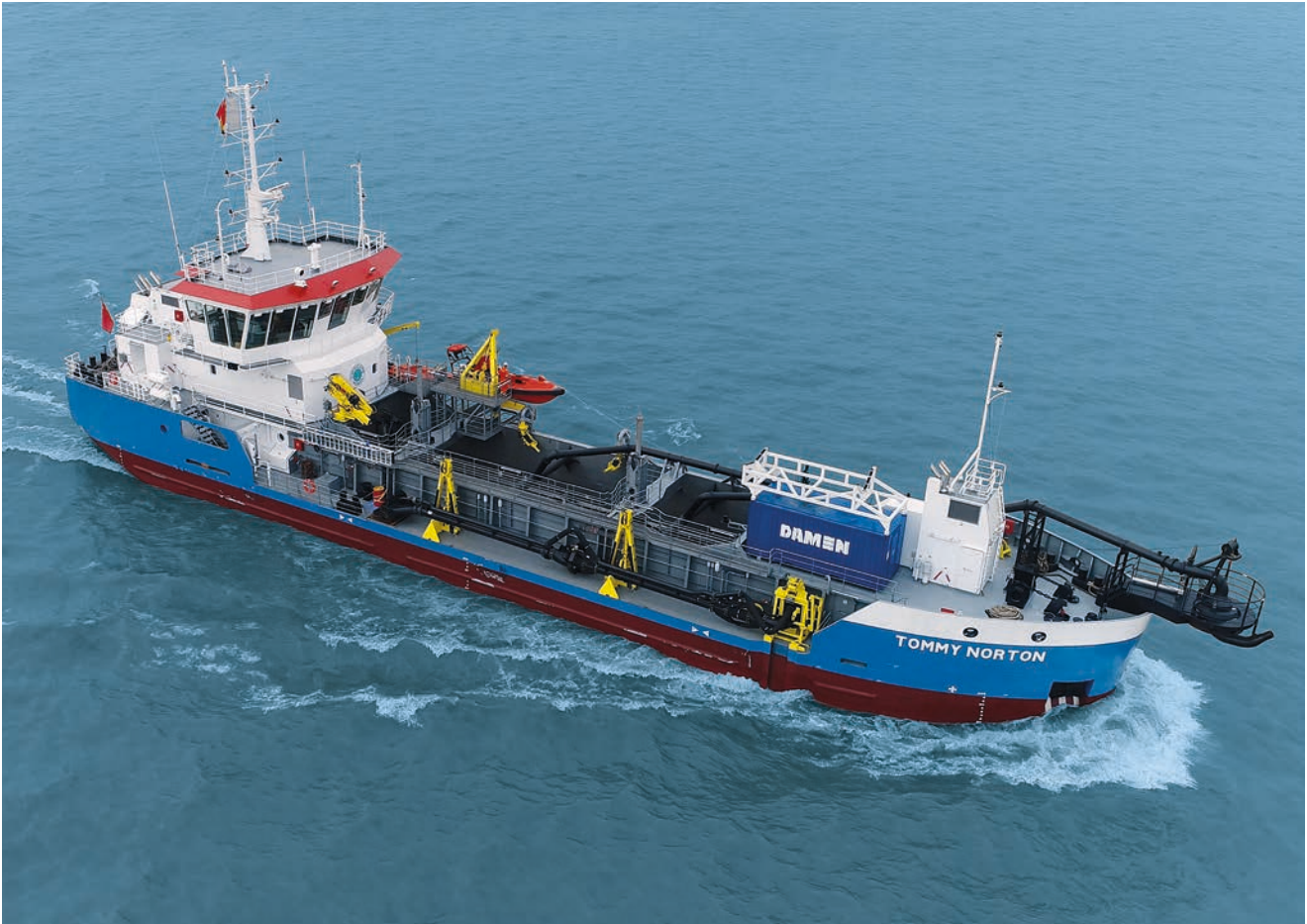
Trailing Suction Hopper Dredger Tommy Norton 2 x SRP 330 (447 kW each)
