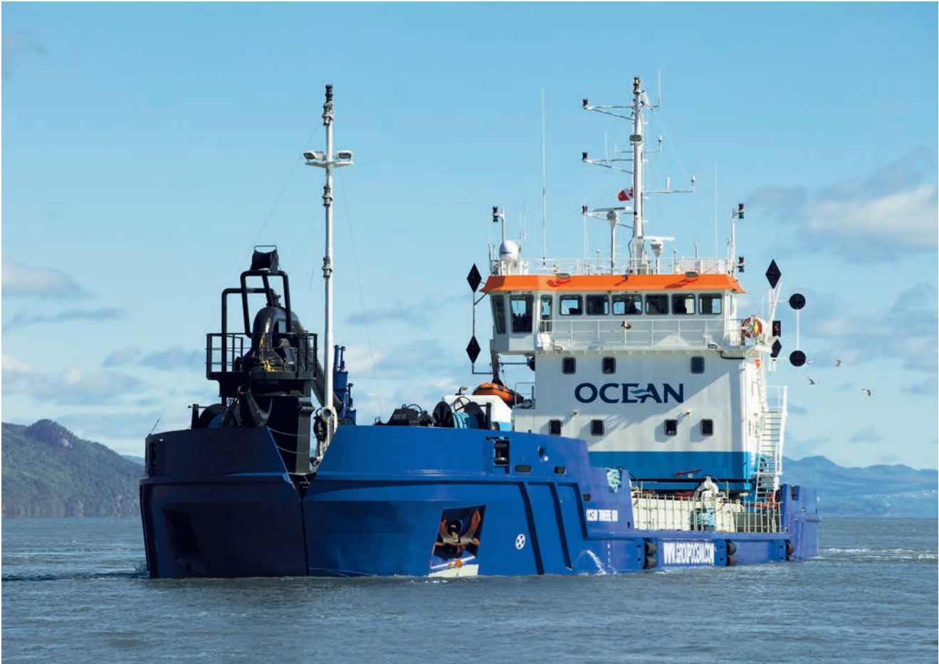
Trailing Suction Hopper Dredger Ocean Traverse Nord 2 x SRP 260 (746 kW each), 1 x STT 170 (224 kW)
