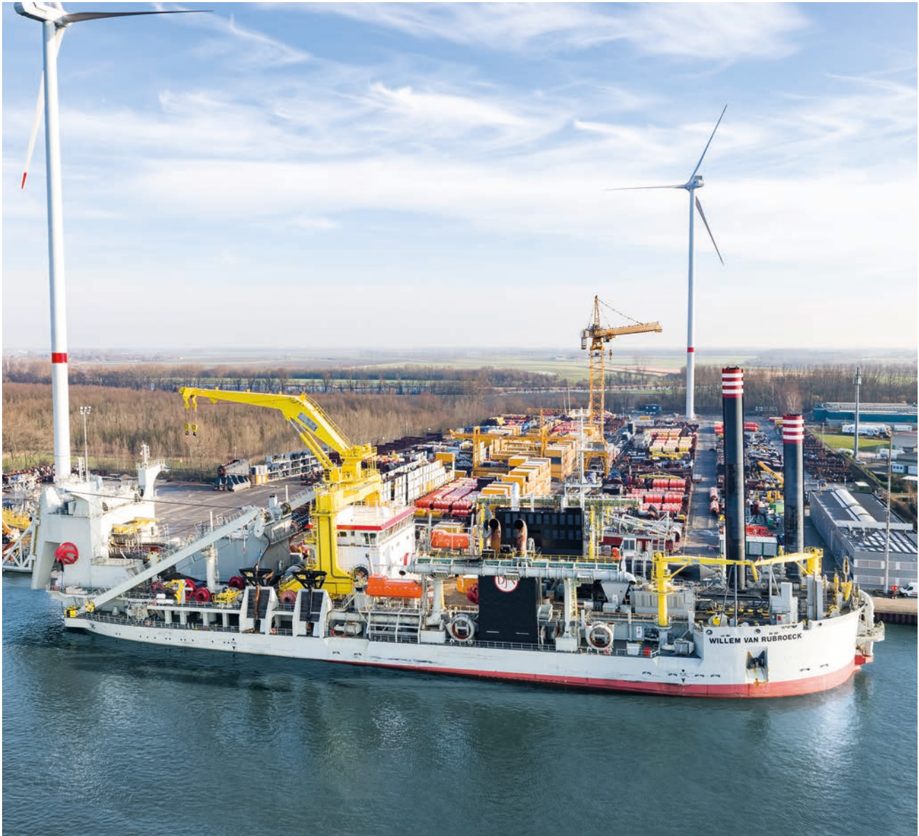
Cutter Suction Dredger Willem van Rubroek 2 x SRP 610 R (3000 kW each), 1 x STT 4 (1200 kW)
