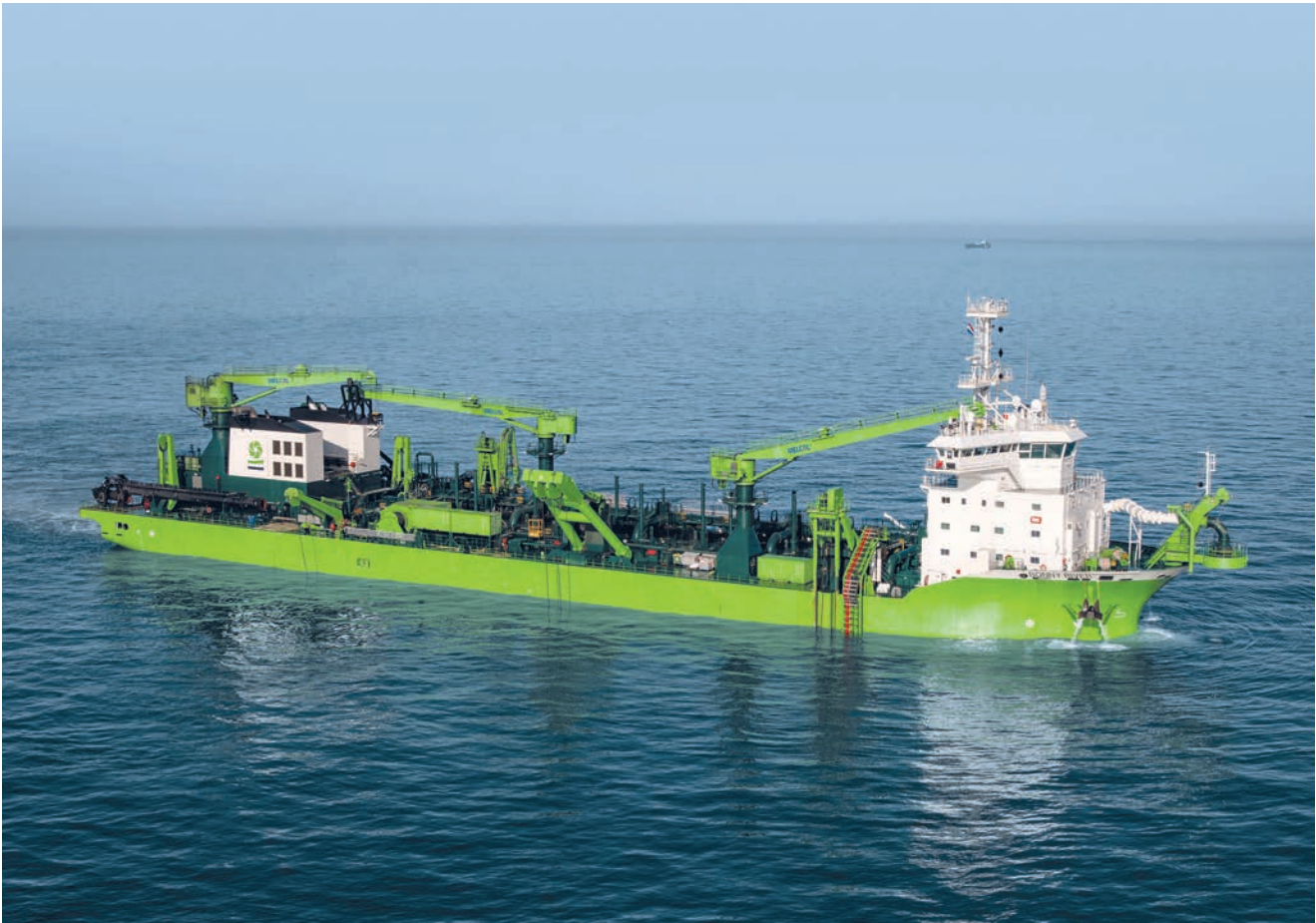
Trailing Suction Hopper Dredger Bonny River 2 x SCP 1294 (8000 kW each), 2 x STT 3 (750 kW each), 1 x STT 5 (1500 kW)
