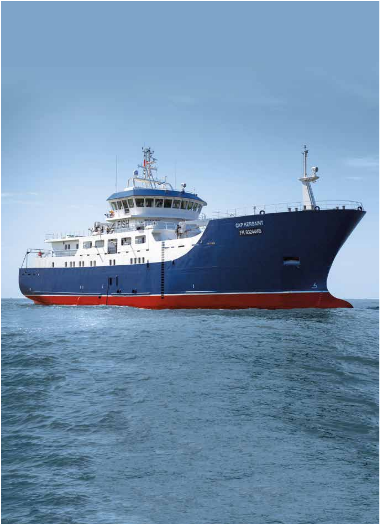
Longliner Cap Kersaint 2 x STP 340 (1000kW each)
