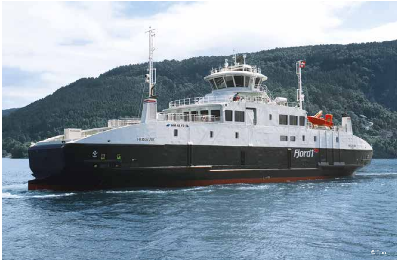
Battery-Powered RoPax Ferry Husavik 2 x SRE 340 CP (900 kW each)
