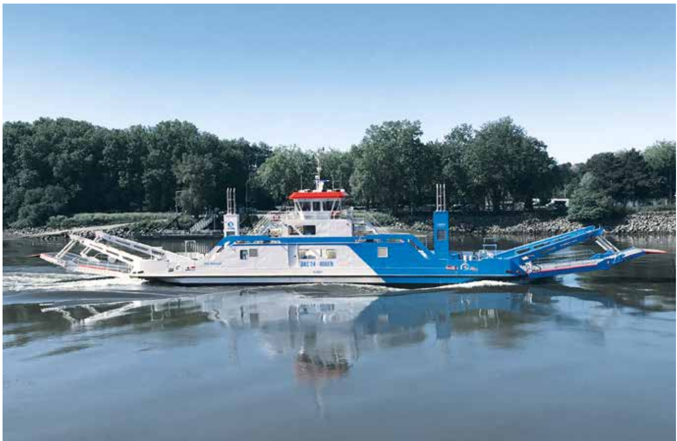
Shallow Water Ferry Bac 24 4 x SPJ 82 (196 kW each)
