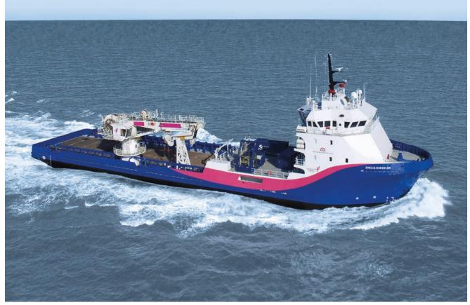
Offshore Support Vessel Shelia Bordelon 2 x SRP 1215 (1641 kW each), 2 x STT 2 (700 kW each)
