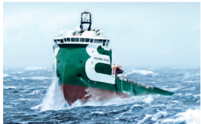
PSV BOURBON MISTRAL 2 x SCHOTTEL Combi Drive Type SCD 2020 (2200 kW each)
