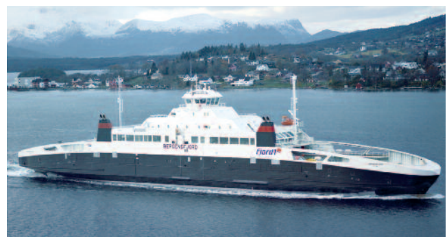
DOUBLE-ENDED FERRY BERGENSFJORD 4 x SCHOTTEL Combi Drive Type SCD 2020 (2750 kW each)
