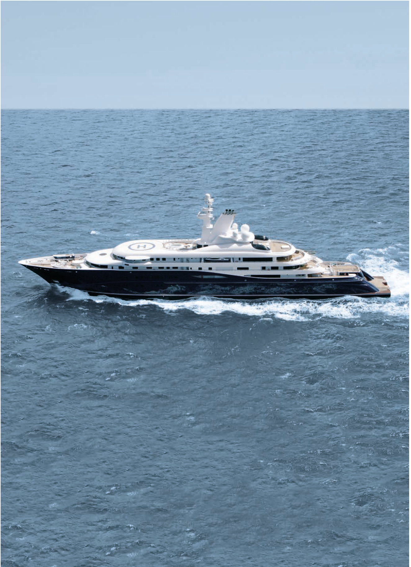
133 m Superyacht AL MIRQUAB 2 x SCP 914 (5,000 kW each), 2 x SPJ 57 (200 kW each)
