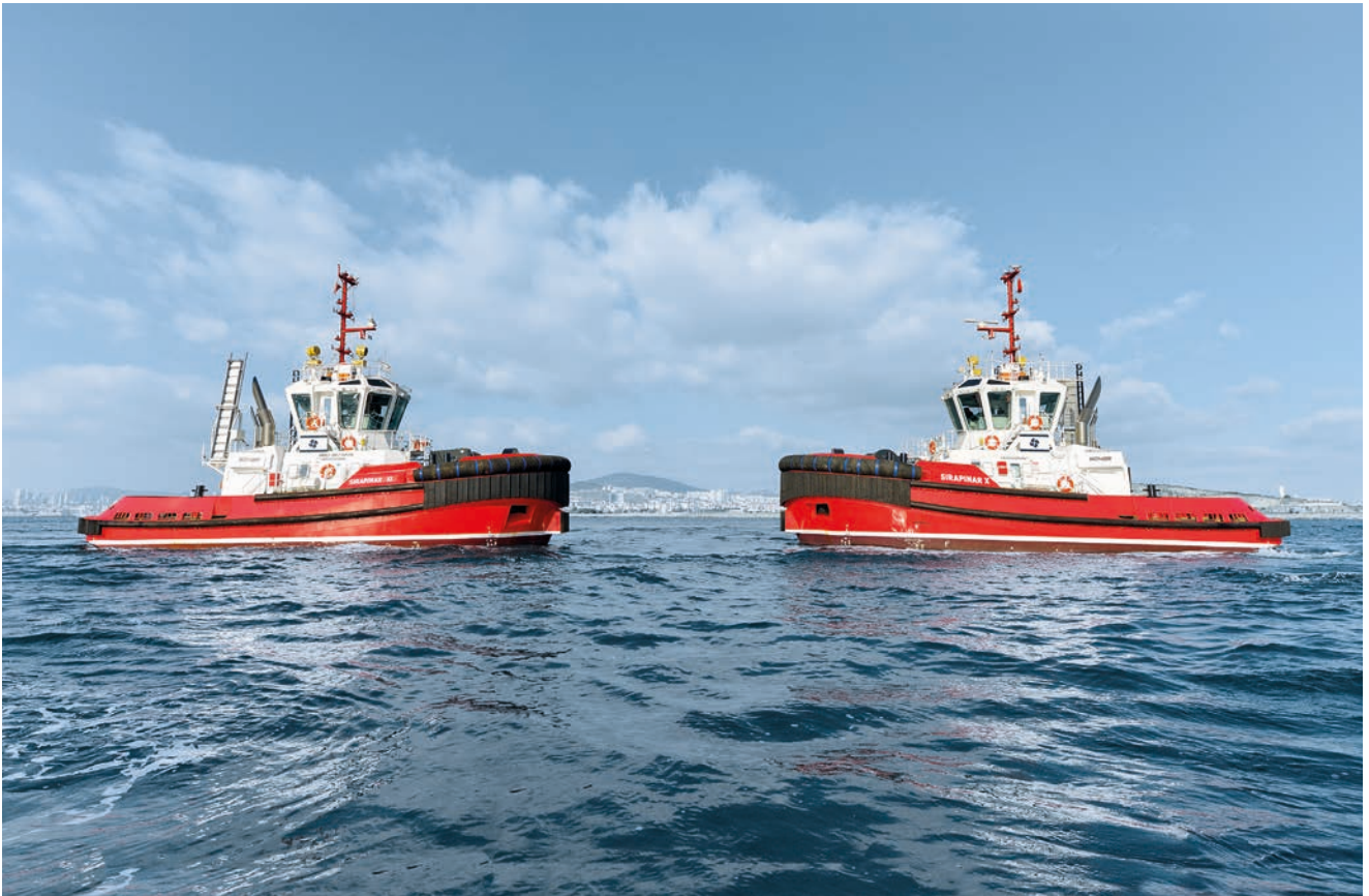
50t BP Harbour Tugs Sirapinar XI, Sirapinar X 2 x SRP 360 (1500 kW each)
