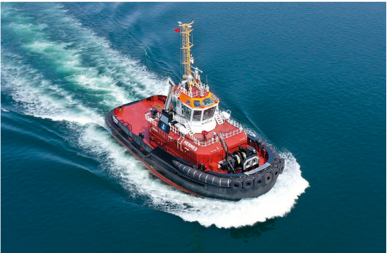
65t BP ASD Tug Hermes 2 x SRP 430 (2000 kW each) with SYDRIVE-M
