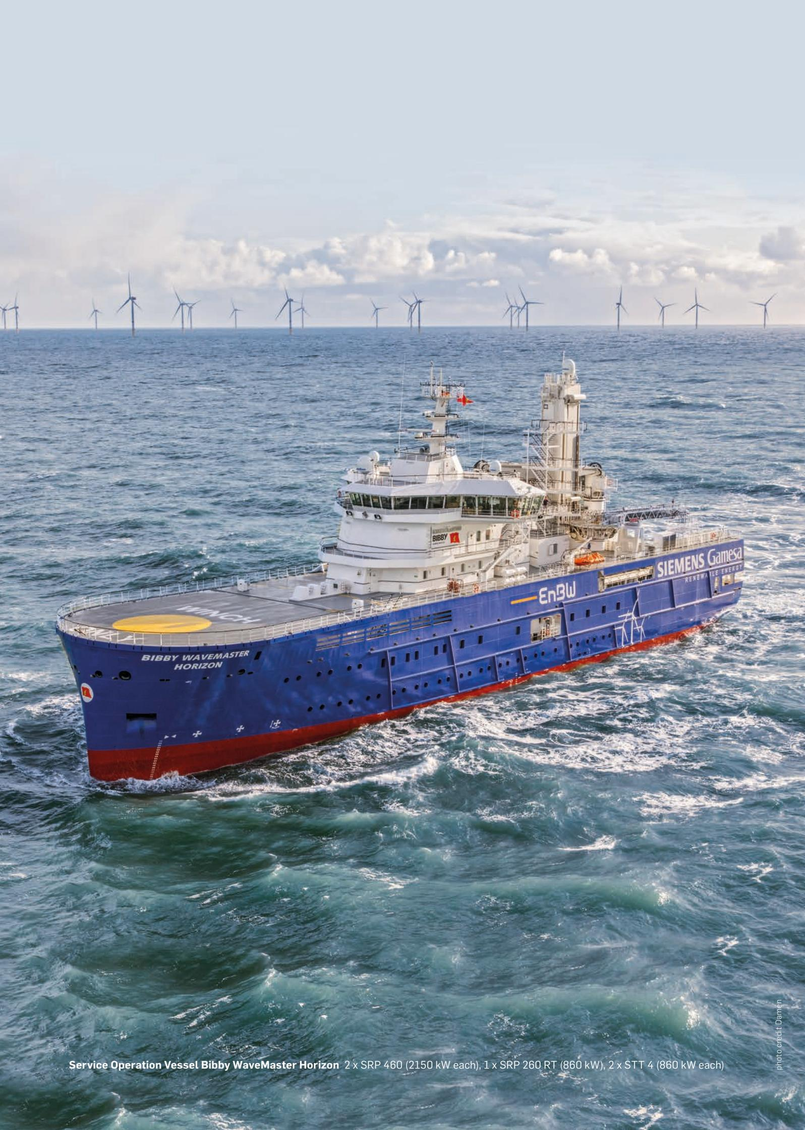
**Service Operation Vessel Bibby WaveMaster Horizon** 2 x SRP 460 (2150 kW each), 1 x SRP 260 RT (860 kW), 2 x STT 4 (860 kW each)
