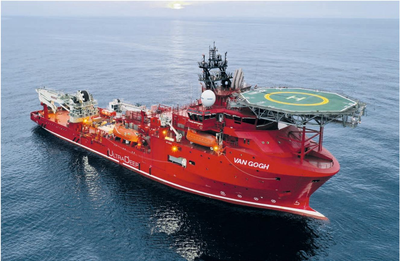
**Diving Support Construction Vessel Van Gogh** 2 x SRP 630 (3000 kW each), 1 x SRP 340 R (1200 kW), 3 x STT 6 CP (1800 kW each)
