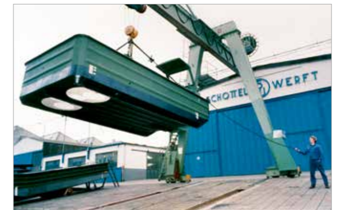
156 M3 boats for the Bundeswehr: a flat bottom and fully protected propulsion units spell enormous success.
