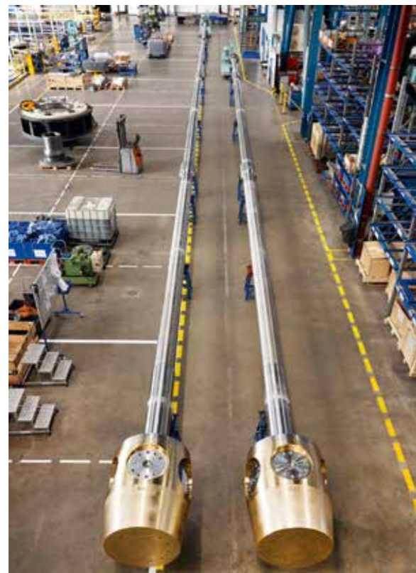
New five-bladed hub, shown here on the left with a 50 metre-long shaft line
