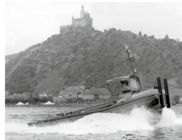
The first two models, the large M-boat and small M-boat (the latter shown here in the picture and in the drawings above), are driven by rudder propellers.
