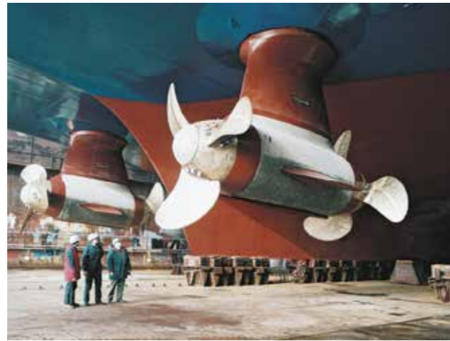
Siemens-SCHOTTEL-Propulsor (SSP), a pod drive with 360-degree rotation and integrated electric motor; here: the ferry Nils Holgersson
