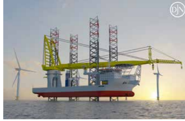
Current offshore reference: with a load capacity of around 14,000 tonnes and a crane capacity of over 3,000 tonnes, the jack-up installation vessel Voltaire will support the renewable energy
